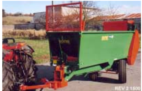
Manure spreader for wine-growers Flared body in one piece
