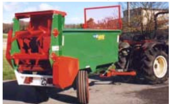
Manure spreader for wine-growers Flared body in one piece
